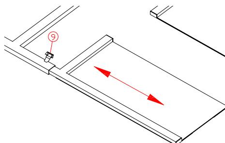
5. **Floor plates:** → Adjustable inwards and outwards by loosening knob (9). Adjust to required position and tighten knob (9).
