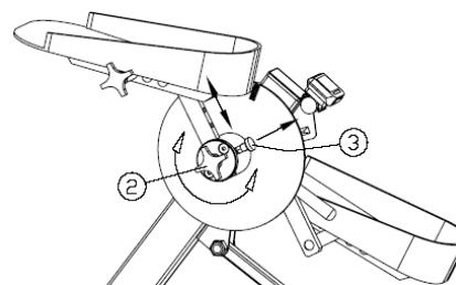
3. Adjusting the pedals: → The crank throw of the pedals may be adjusted by first loosening the knob (2). Pull out the lockpin (3) and push or pull the pedal to the required position. Make sure that the lockpin (3) lines up with a hole and replace the lockpin. Tighten the knob (2).
