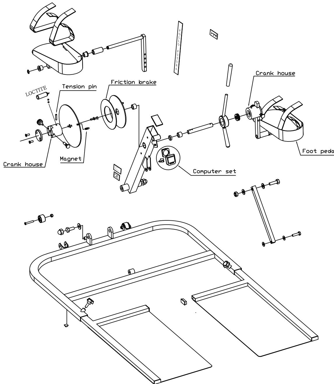
1. Check the friction brake and if it is worn, change it.
