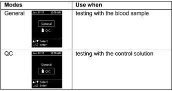
You can switch between each mode by: In the measuring mode, after a test strip is inserted, press  $\blacktriangle$  or  $\triangledown$  to select a suitable measuring mode when the meter displays the list. Press **M** and proceed with a lactate testing.
